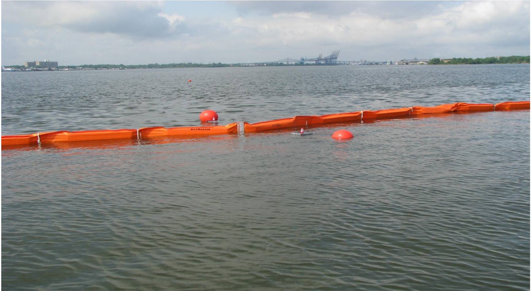
Figure 3-1. The initial configuration of the curtain. The curtain boom is anchored in place but the curtain is not unfurled.
